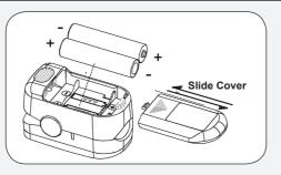
Please put in the batteries according to the polarity marked inside the battery compartment.
