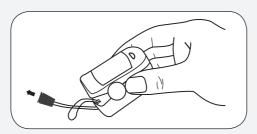
Tie the lanyard through the hole in the rear of the pulse oximeter.
