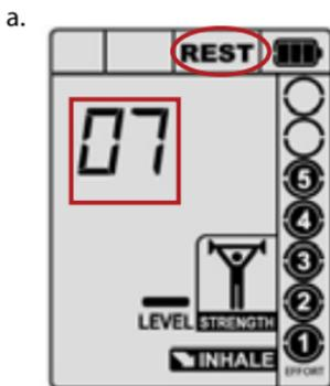
In this example, the user inhaled in strength mode at level one at an effort of 5.
